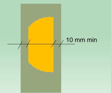
Max 20 % of X sect, and max ½ width of face and ½ thickness
